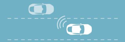
Blind Spot Assist Pack (Optional<sup>9</sup>) can help you prevent collisions. If another car is in your blind spot when you begin to change lanes, Blind Spot Assist detects the car and applies corrective torque to encourage you to guide your vehicle away from the approaching vehicle. Rear Traffic Monitor uses the same system to alert you, via the Touchscreen, of moving vehicles during reversing.
