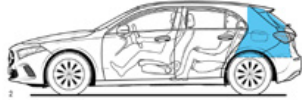
2 Open luggage compartment behind rear seat, loaded to roof, volume 375 litres (V 214-2)
